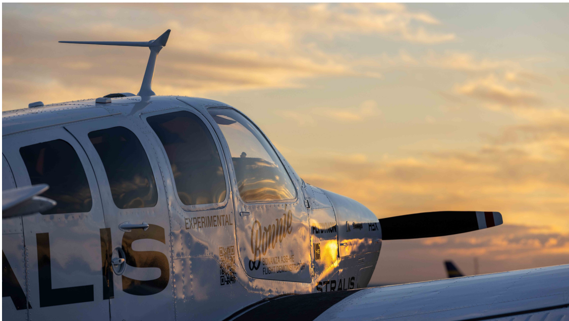
Bonnie — a hydrogen-electric Beechcraft Bonanza A36 — airside at Brisbane Airport. Photo Steven Holden.
